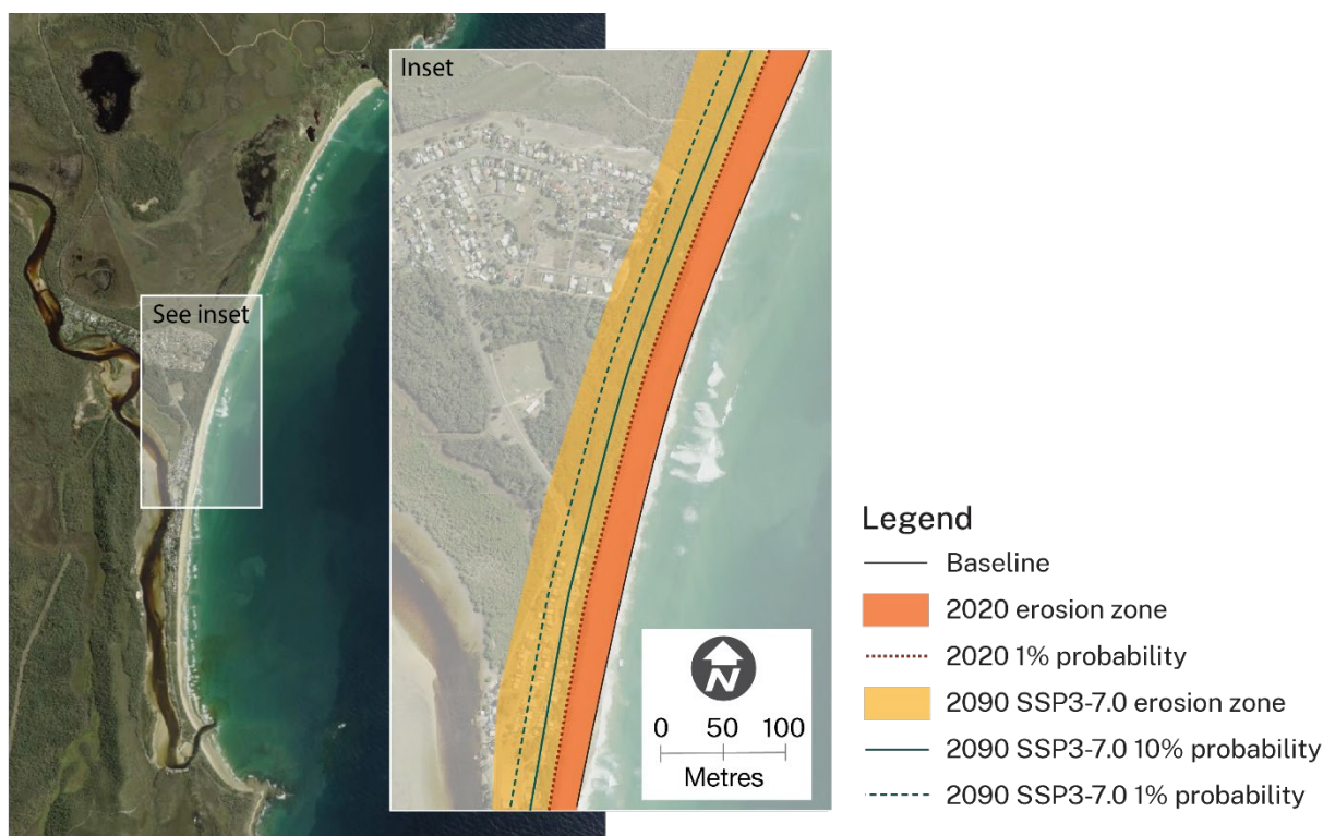
Figure 11 Coastal erosion mapping for Woolli Beach showing the modelled potential erosion extent at present (2020) and for the SSP3-7.0 scenario in 2090
