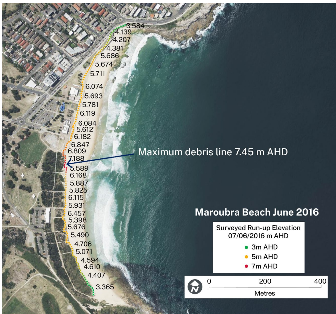
Figure 5 Surveyed debris line on Maroubra Beach (Sydney NSW) on 7 June 2016 showing inundation elevations (m AHD) following the June 2016 east coast low
