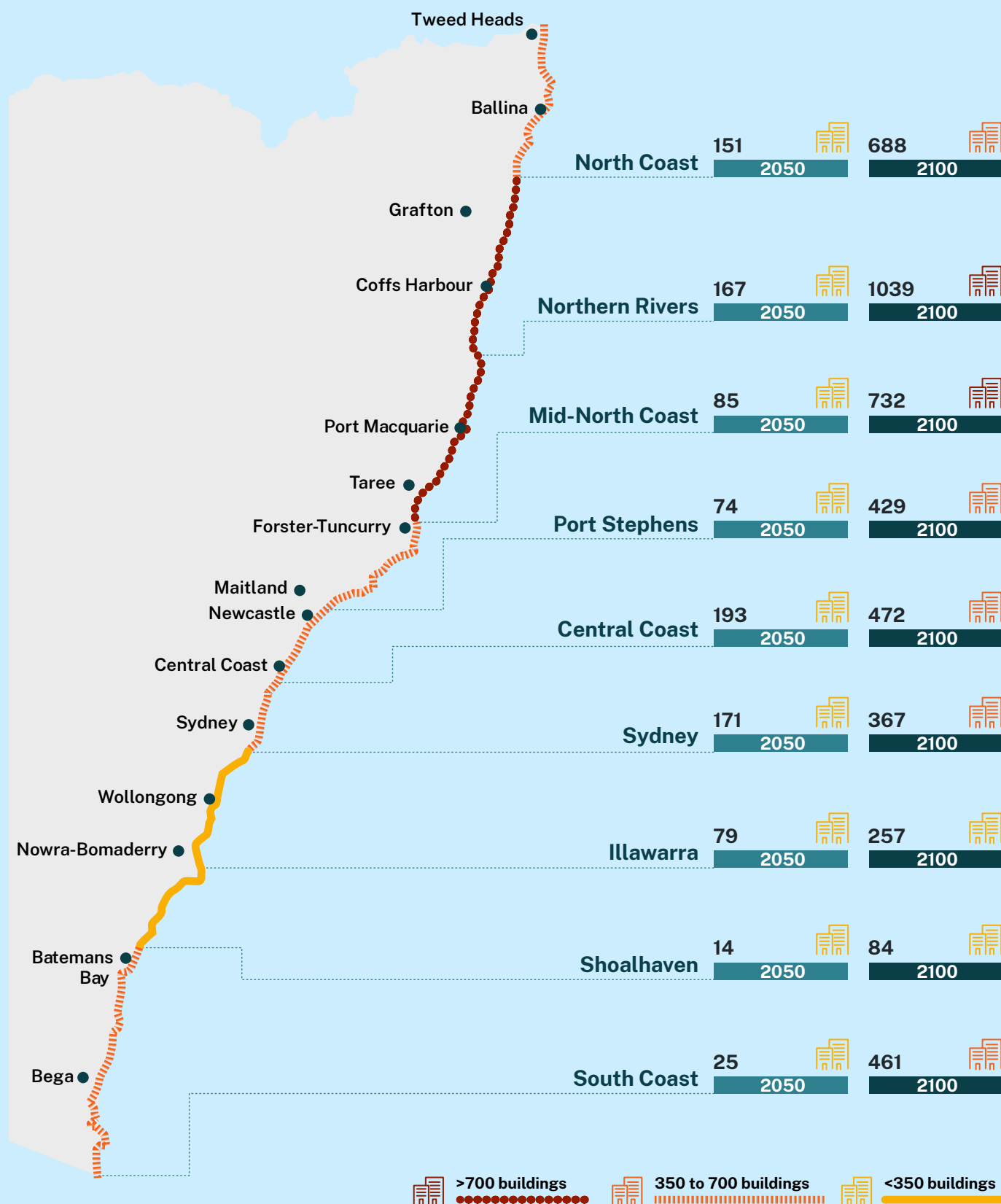
Figure 7: Map showing the nine primary sediment compartment regions along the NSW coast and the number of buildings exposed to coastal erosion at 1% probability level, under a high-emissions scenario (SSP3-7.0) at 2050 and 2100. NOTE: Multiple building categories were included in the analysis; therefore, the building exposure results presented here do not represent a single building class.
