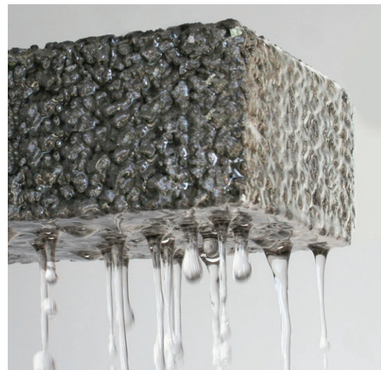
Water infiltration through permeable paving units – Hydroston permeable paver (HydroCon Australasia hydroston.com.au )
